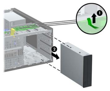
• To remove a hard drive from and internal 3.5-inch drive bay, pull up on the green hard drive drivelock mechanism (1) for that drive and slide the drive from the drive bay (2).
